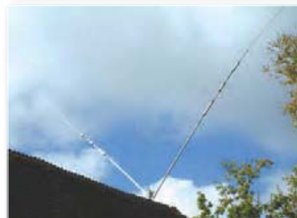
Fig. 10: The Comet H422 rotary trapped dipole (used in a V form in this photograph) antenna for 7, 14, 21 and 28MHz. It can be used either 'flat' ordinary dipole form) or in the V form as shown.
